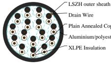
Drain Wire Plain Annealed Copper Aluminium/polyester tape XLPE Insulation
